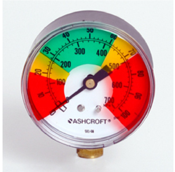
FIGURE 1. GAUGE INDICATIONS OF CATEGORIES OF CONCERN. THE GREEN AREA OF THE GAUGE (200-400 KPA) REPRESENTS NORMAL OPERATING CONDITIONS. THE YELLOW AREAS OF THE GAUGE (100-200KPA, 400-500 KPA) REPRESENT AN AREA OF LOW CONCERN. THE AREAS OF RED ON THE GAUGE (0-100 KPA, 500-700KPA) REPRESENT AREAS OF HIGH CONCERN. AREAS BEYOND THE HIGH AREAS OF CONCERN REPRESENT AREAS OF FAILURE CONCERN.
