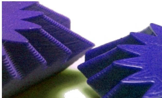
FIGURE 13. Bevel gears manufactured from PLA using FFF in the "as printed" state (at left), and after a 10-second exposure to ethyl acetate vapor at 115 °C (right).
