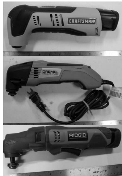
Figure 2. THE INNOVATIVE RIDGID JobMax™ (BOTTOM) IS COMPARED TO THE Dremel® Multi-Max™ (MIDDLE) AND Craftsman® Nextec Multi-Tool (TOP).
