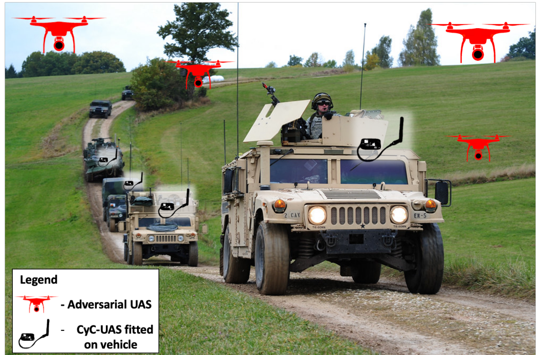
Figure 8. CONOPS of ground mobile defensive deployment of CyC-UAS to protect vehicles and civilians.
