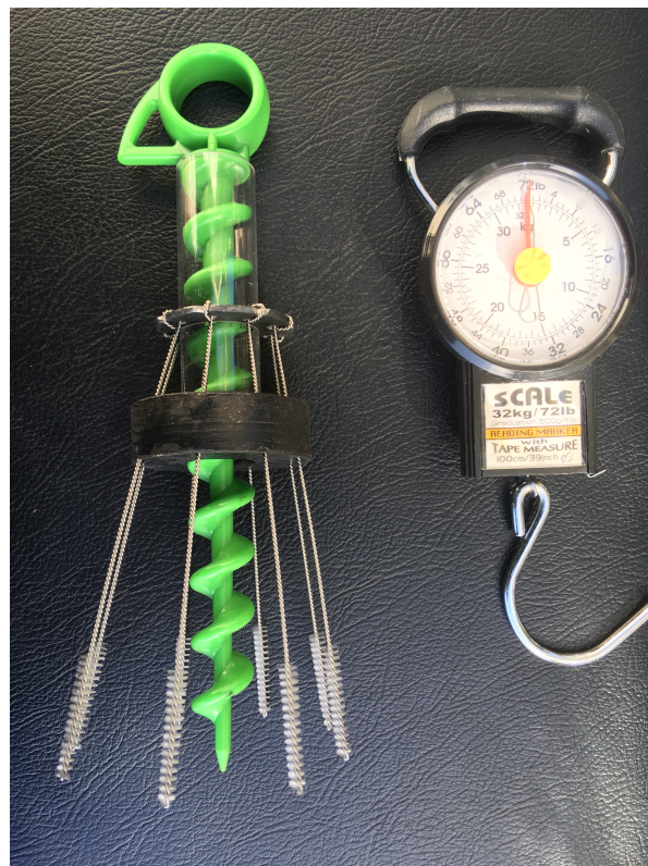
Figure 12. The RAATM anchoring strength test prototype and scale.
