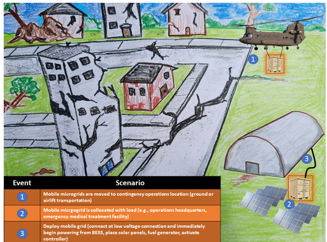
Figure 4. This CONOPS for contingency operations shows a mobile microgrid being airlifted to the contingency environment and collocated with an operations headquarters. The load can be powered from the BESS immediately after the mobile microgrid is dropped at the site. Workers can then position the PV array while the load is powered with the BESS, within safety requirements, because the mobile microgrid is a low voltage (48 V) system.
