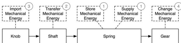
**Fig. 5 Clock energy chain component selection**
