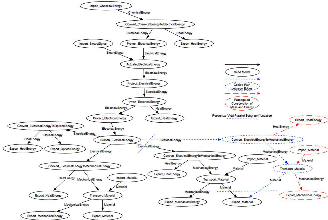
Fig. 3 Functional model of electrical power system
