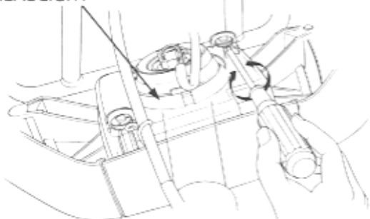
VIEW FROM UNDER THE FRONT COWL: (1) HEADLIGHT
