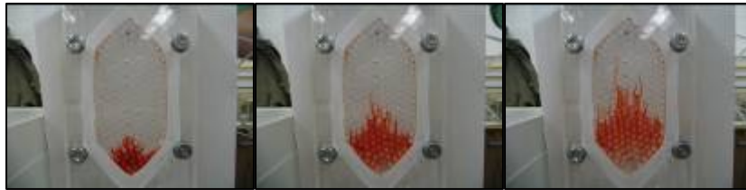
Figure 14 Flow Developing Into Right, Center, and Left Regions
