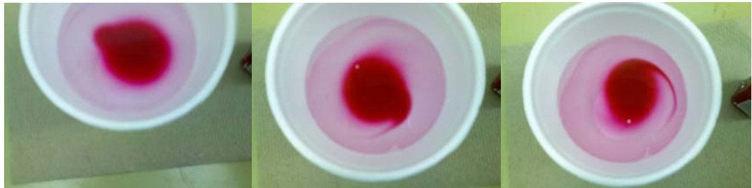
Figure 10: Oil Paint Dye Test (8 second time intervals from left to right)
